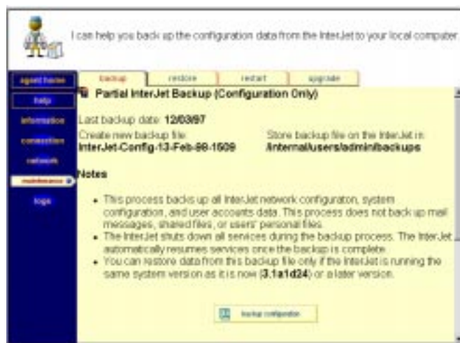
Figure 7-19 The Maintenance Backup page
